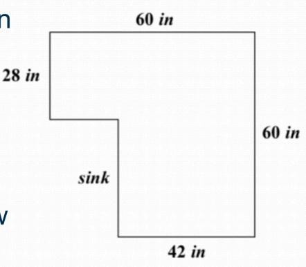
This diagram of the bathroom floor shows the dimensions of the floor space she needs to cover. The sink area does not get tiled.
