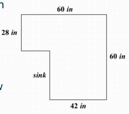
This diagram of the bathroom floor shows the dimensions of the floor space she needs to cover. The sink area does not get tiled.
